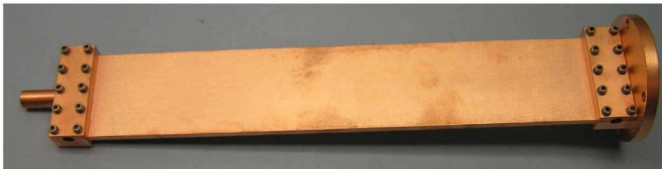
Figure 1. Copper conduction bar - attaches to the sensor thermal manifold on the left, and Cryomech cold heat exchanger on the right.
