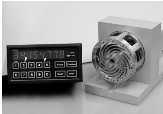
Figure 2: Nine-finger spiral flexure endurance test setup. Over 1.1 trillion cycles (>8 years) accumulated without failure. Flexures of this design have been used for several Raytheon cryocooler programs. (Counter shown rolls over every 26 days, so actual accumulated run time is tracked with the log book.)
