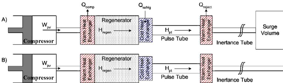
**Figure 1.** Schematics of modeled PTRs; (A) Inertance Tube PTR, (B) Reservoirless Inertance Tube PTR.
